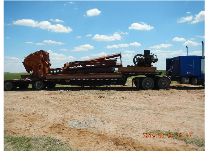
Photo 6: Flatbed trailer loaded with pumping unit.
