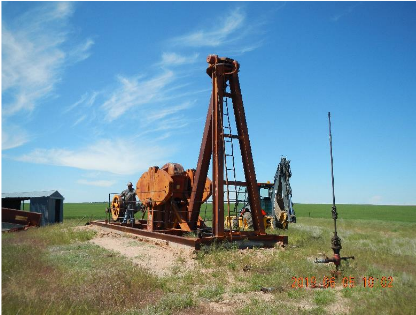
Photo 1: Pumping unit with horsehead and walking beam removed.
