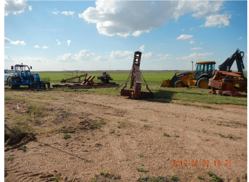
Photo 10: Disassembled pumping unit ready for loading.
