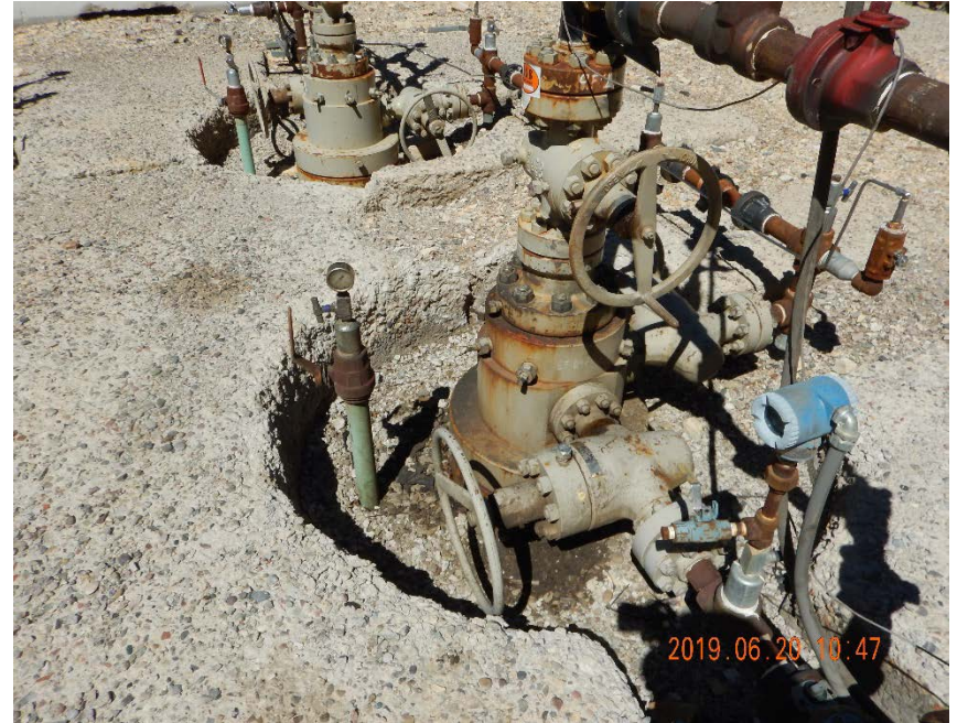
Photo #12 - NP EF09F-27 P27 595 wellhead with oil-stained material.
