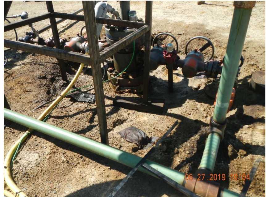
Photo 8. Stained soil at wellhead, oily rags and trash at wellhead.
