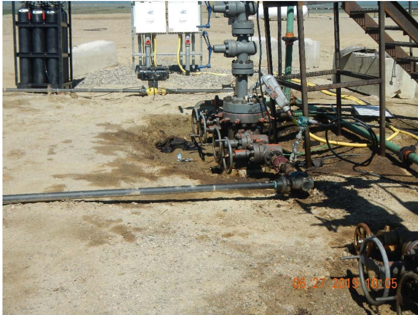
Photo 9. Stained soil at wellheads, oil rags and trash and wellheads.
