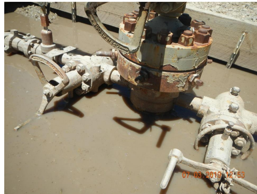
Bubbling around well head GM 44-20
