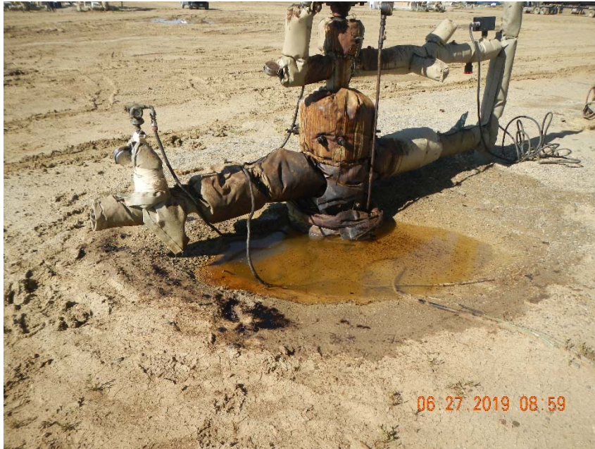
Photo 9. Cellar full of stormwater with free product on top and stained soil around wellhead.
