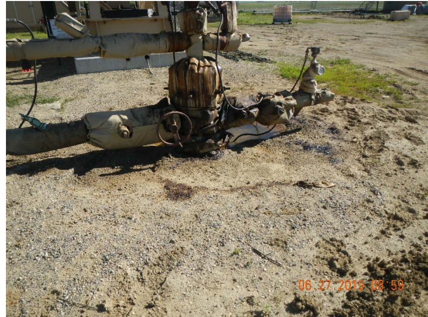
Photo 8. Cellar full of stormwater with free product on top and stained soil around wellhead.
