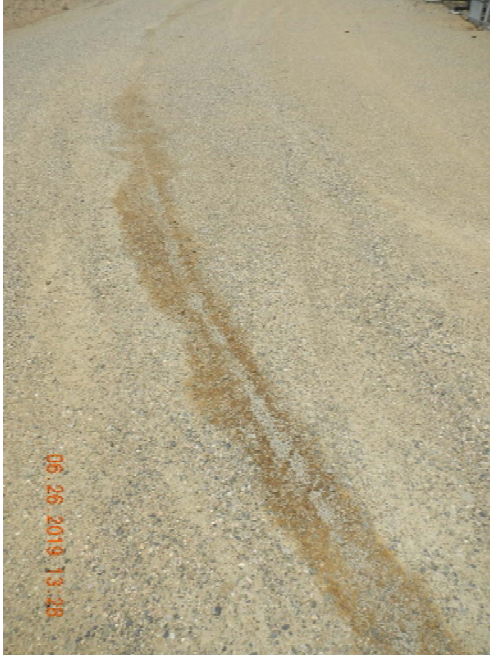
Photo 3. Close up of hose drag soil staining.
