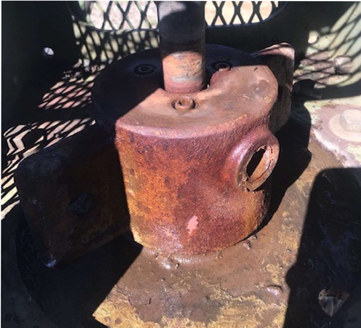
PHOTO (1): APACHE CANYON 14-10 WELLHEAD PACKINGS REPAIRED TO STOP THE WATER LEAK.
