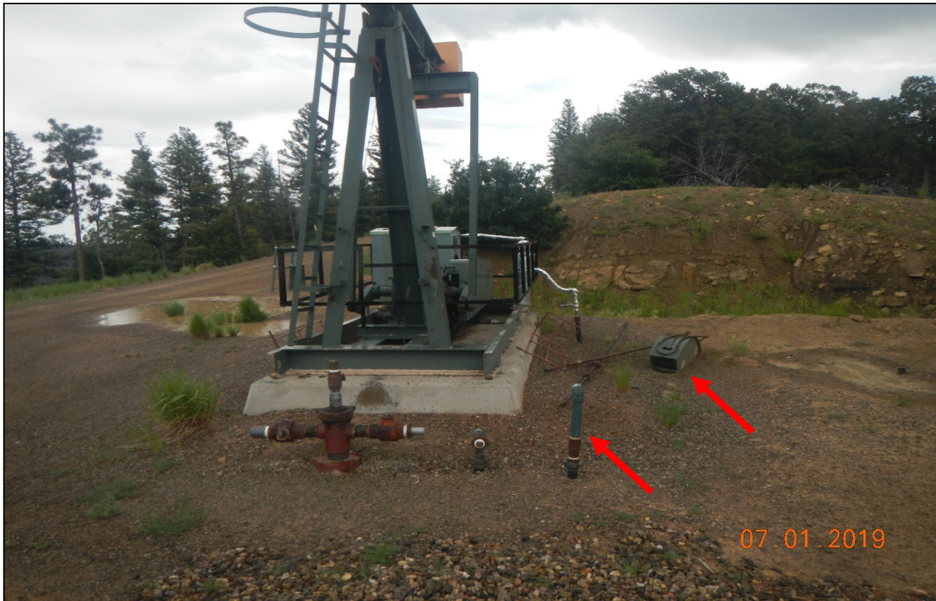
Photo 4. Facing toward pumpjack. Unused equipment remains. Pipe risers with not LO/TO are unused equipment.
