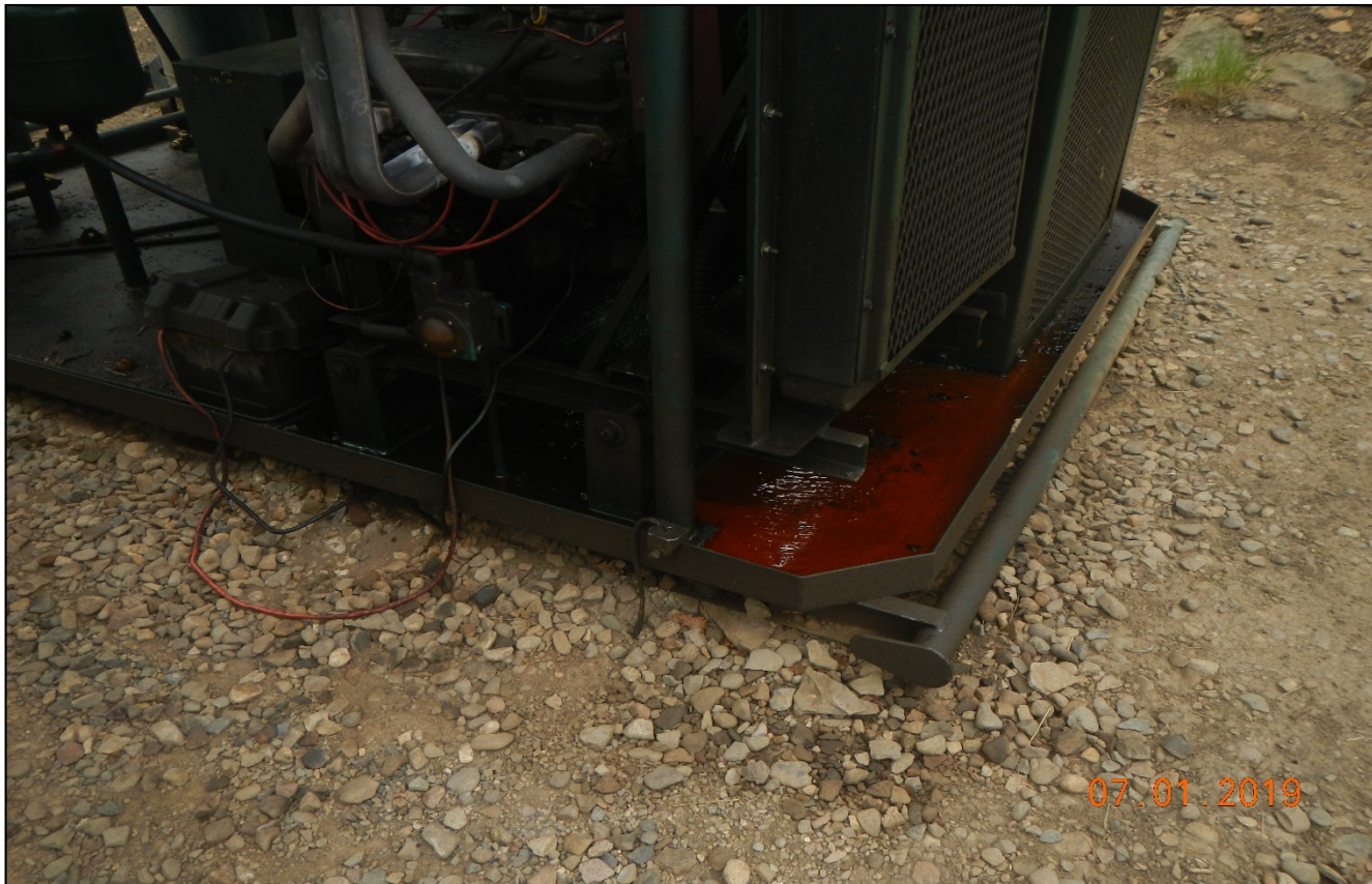
Photo 5. The oily waste has not been cleaned up since previous inspection.
