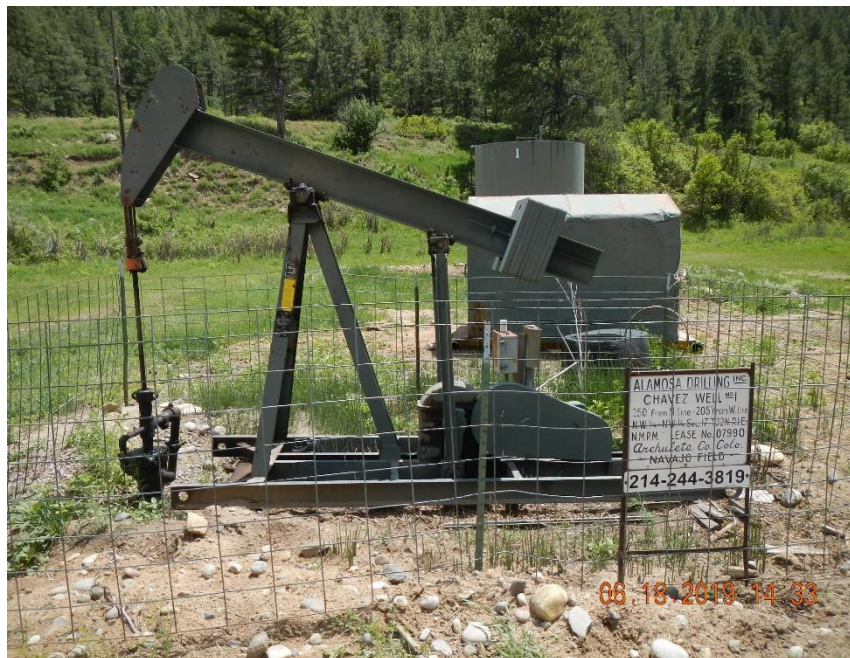
Chavez #1 pump jack and well head.
