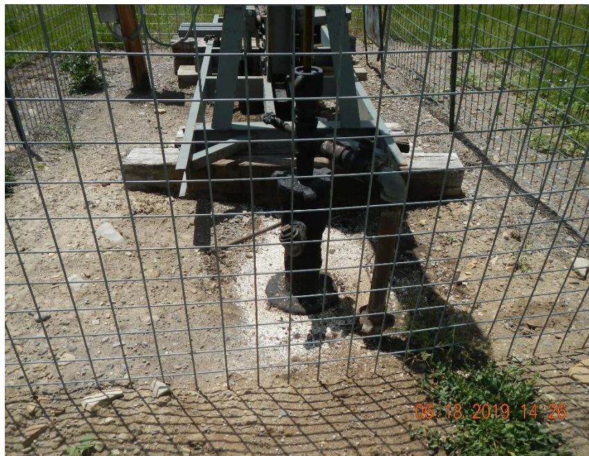
Absorbent granules observed around the well head during this inspection.
