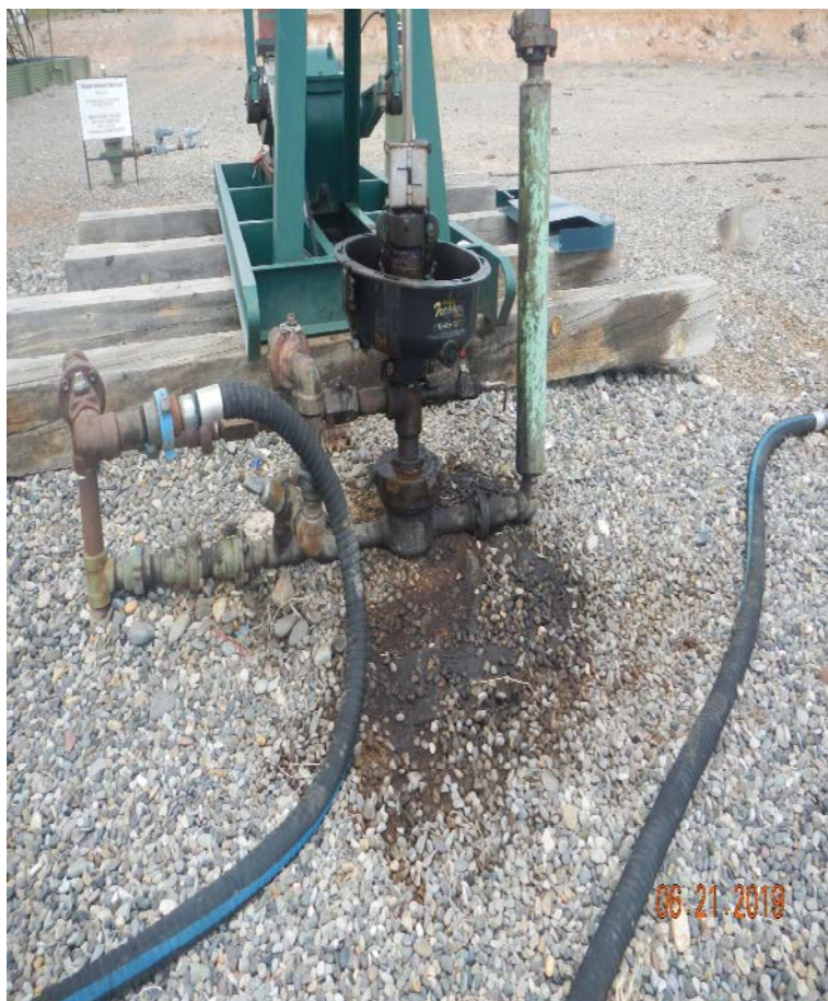
Photo#4: Stained soil and equipment coated with oily waste.
