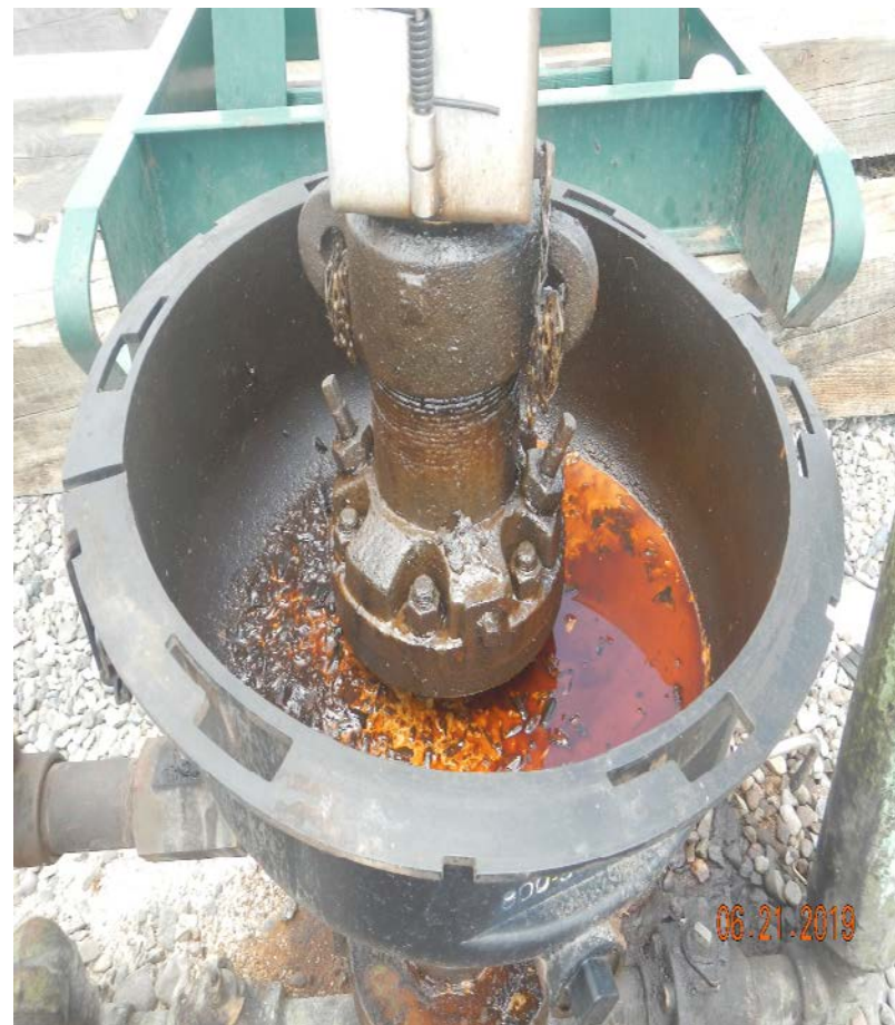
Photo#5: Stained soil and equipment coated with oily waste.
