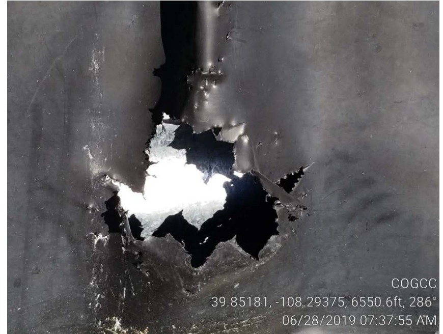
Photo 4. Hole in tank secondary containment liner.
