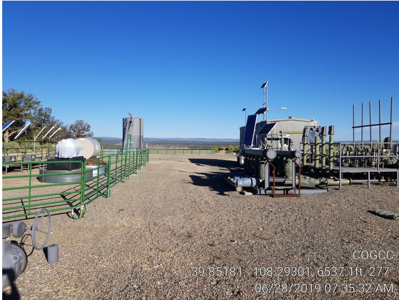
Photo 2. Header, separator, tank, chemical totes.
