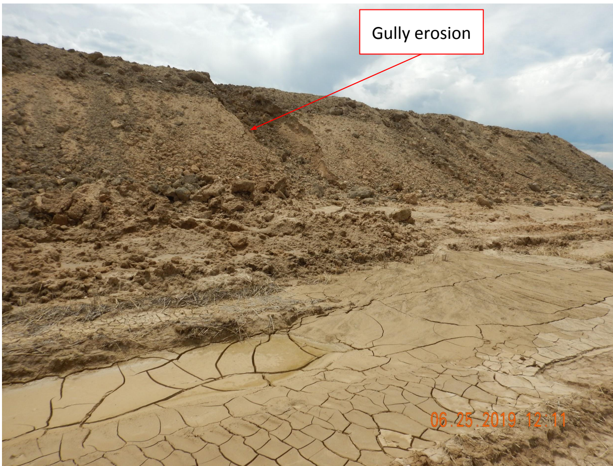
Photo 9. Photo taken from northwestern perimeter of location, facing Southwest. Photo illustrates gully erosion along the fill slope which has filled in the perimeter ditch and berm BMP.
