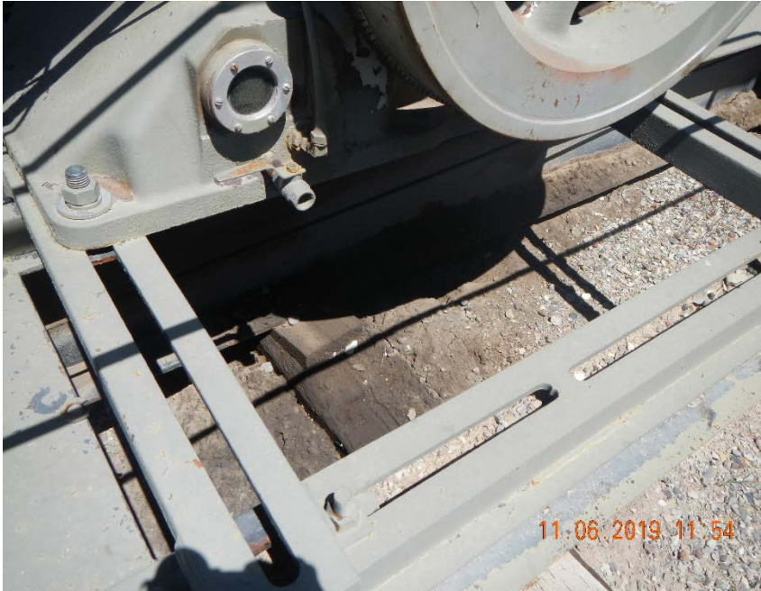
Photo #5 – Accumulation of oil-stained soil beneath prime mover.
