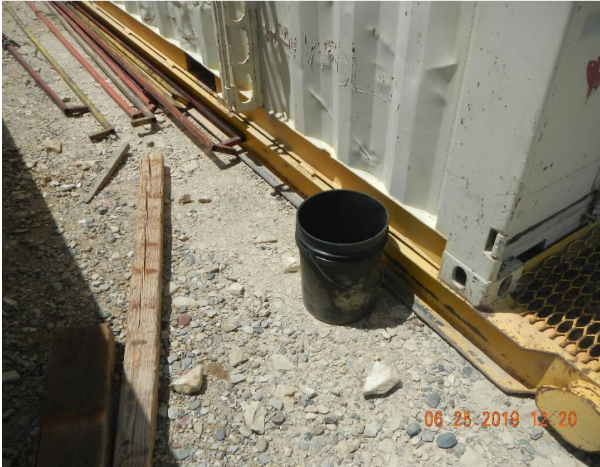
Unlabeled 5 gallon bucket by diesel tank has no secondary containment..
