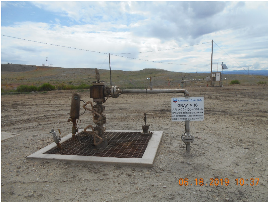
Injection wellhead
