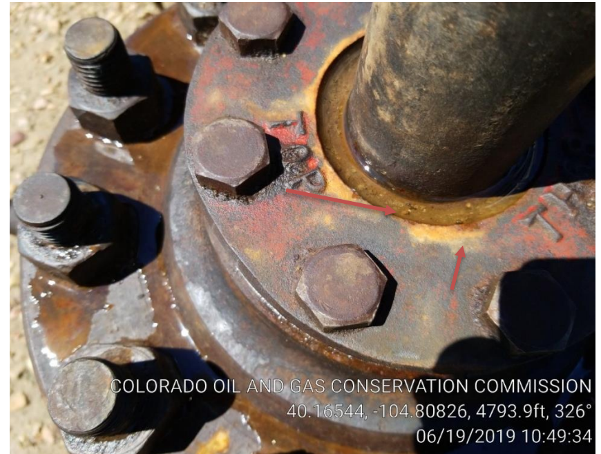
Pic 4 bubbles coming out of packing
