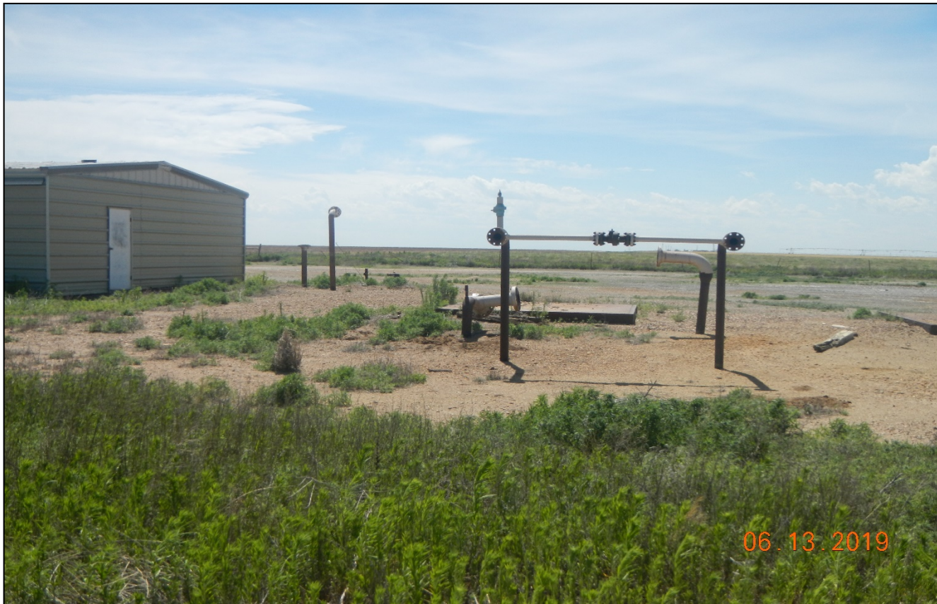
Photo 8. There is numerous abandoned pipe risers at the east side of the location.
