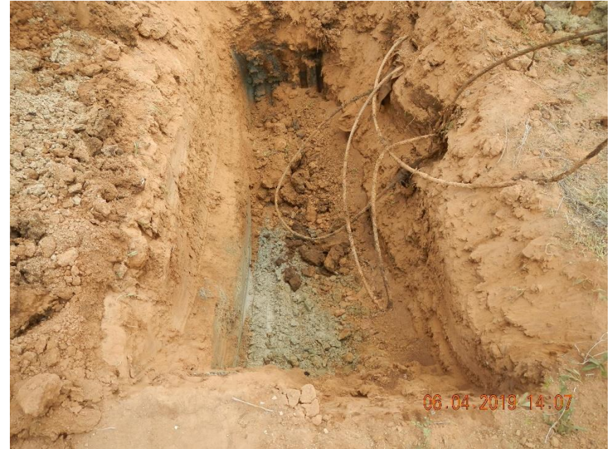
Grayish blue material with strong hydrocarbon odor discovered at depth.
