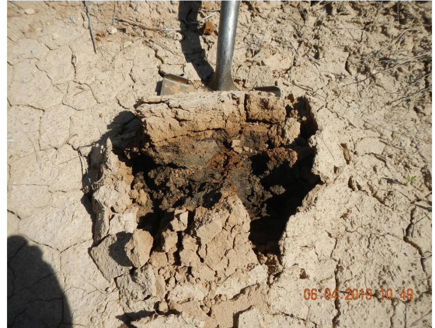
Impacted material below the surface of dry portion of pit.
