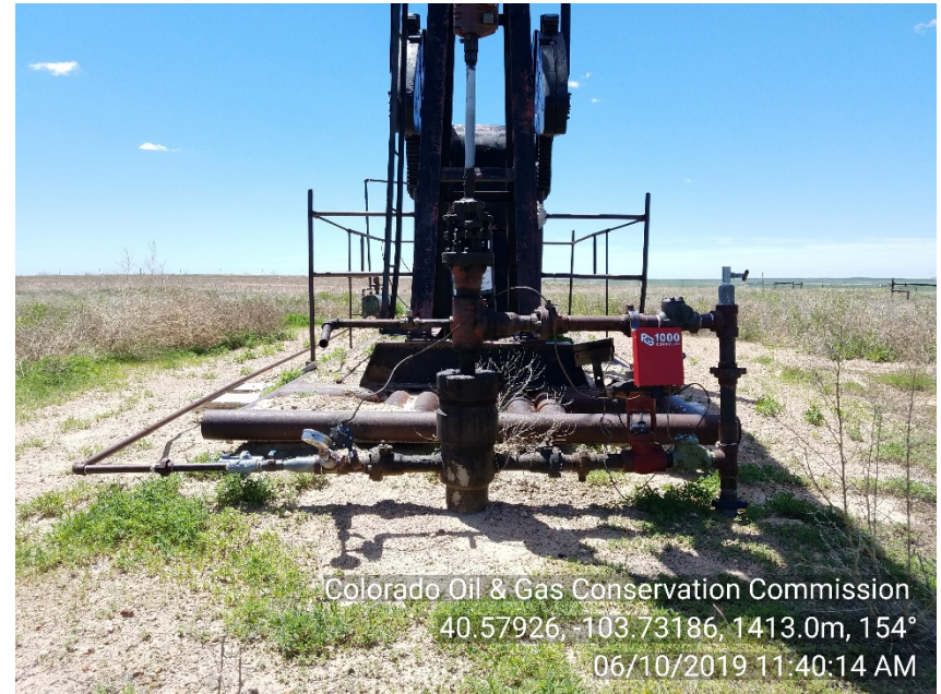
Photo #2 Chinook #1 Wellhead Shut-In | SI Weeds Bradenhead NOT plumbed to surface
