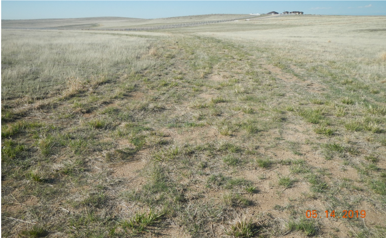
Photo 12. Facing south toward the reclaimed access road and location. Vegetation appears to be establishing. This photo depicts compliance of the corrective action.
