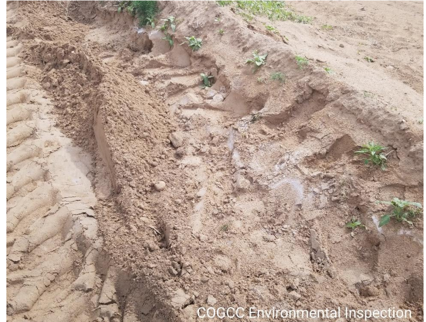
Photo 2 - Salt crust observed on surface soil adjacent to the hydrovac excavation. During site assessment Operator shall characterize impacts to top 0-6" in addition to subsurface impacts.
