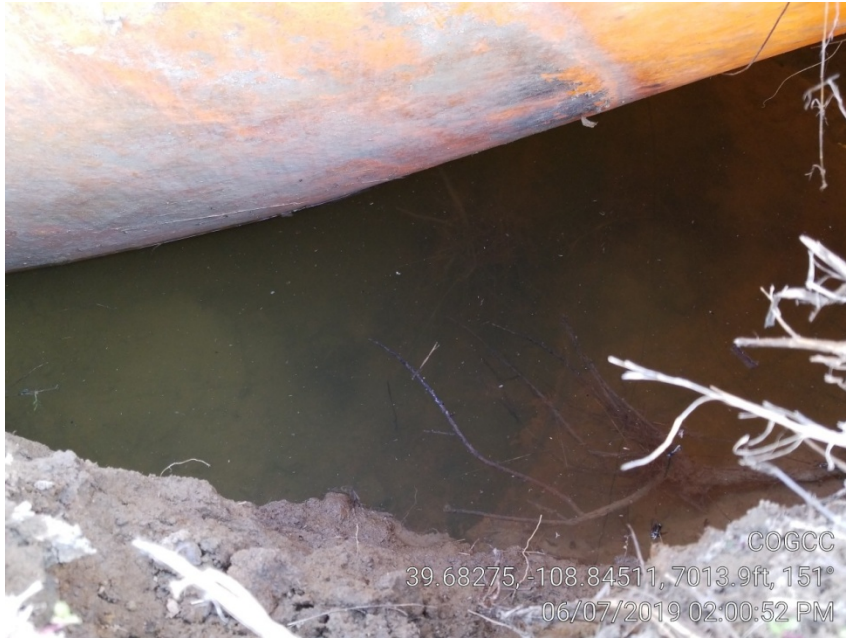
Photo 6. Fluid in hole created when tank tilted over.
