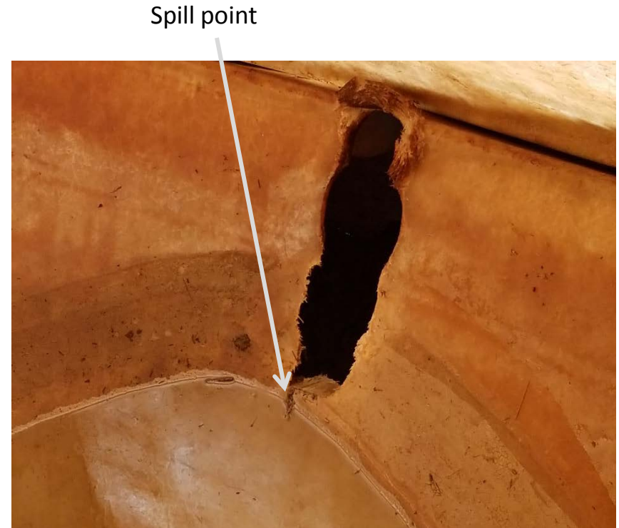
Photo 7. Inside of tank. Top of fluid at spill point of hole.
