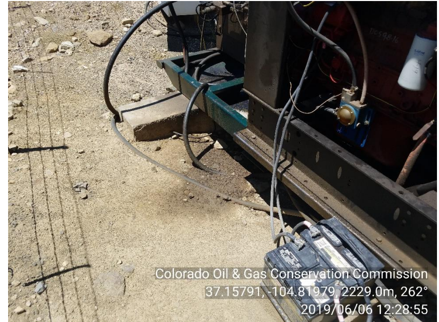
PHOTO 3: AREA OF IMPACTED SOIL APP. 2' BY 2' ON EAST SIDE OF ENGINE SKID AND PUMPJACK. Remove and dispose impacted material in approved manner, service and maintain equipment and self inspect to prevent recurrence of conditions per 1002.f(2) and 907. CA DATE 7/6/19.
