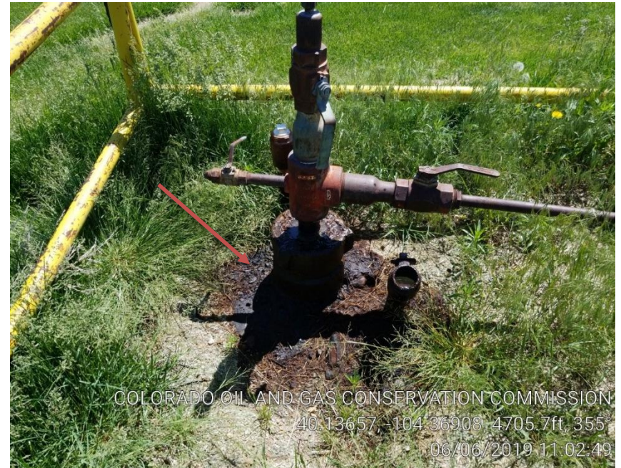
Pic 2 stained soil/possible leak
