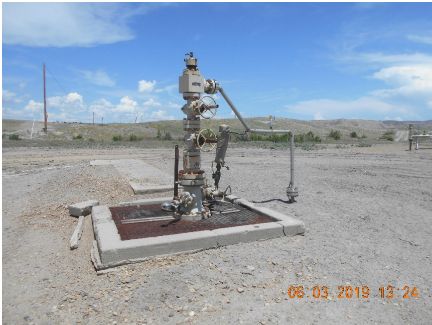
Injection wellhead
