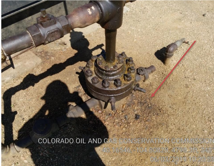
Pic 3 Stained soil/possible leak
