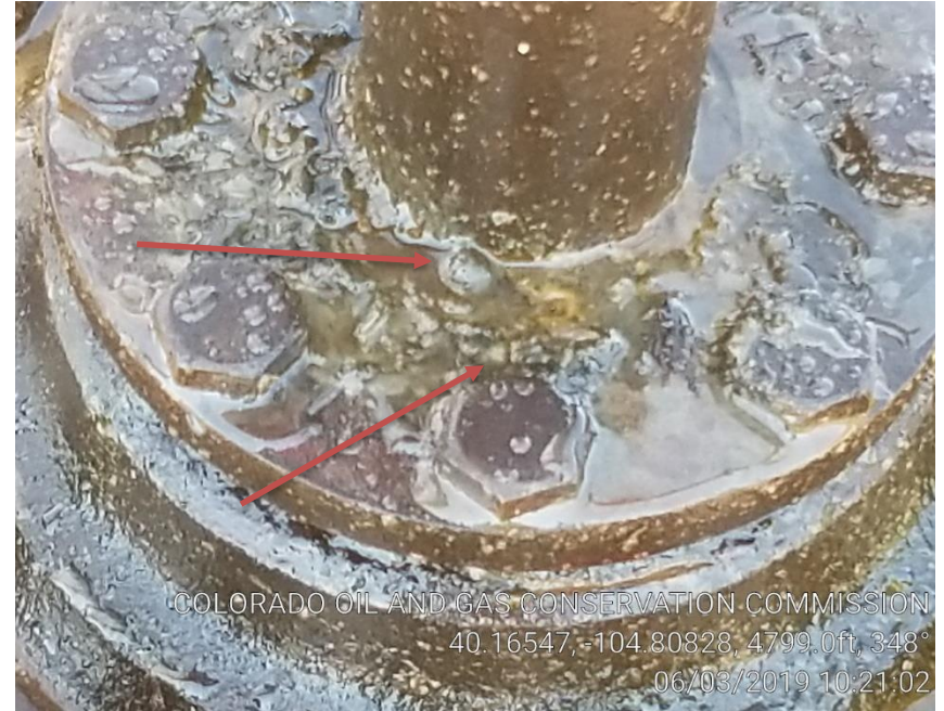
Pic 4 Bubbles on wellhead
