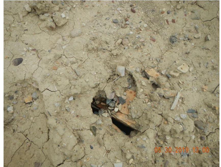
Rathole has subsided and is exposed.
