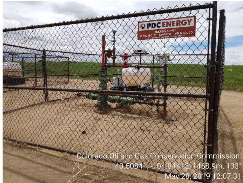
Photo 1: Wellhead w/methanol pump
