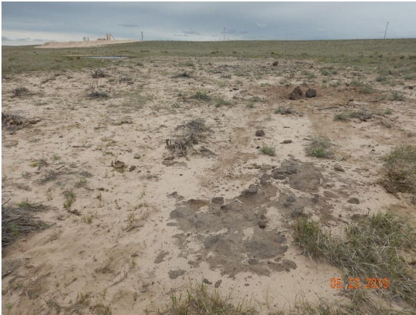
Photo 9: Photo taken from the east of the pits, facing northeast. Photo shows unvegetated areas where stained/contaminated soils are also evident. Aerial imagery suggests possible historic spill or discharge from pits.
