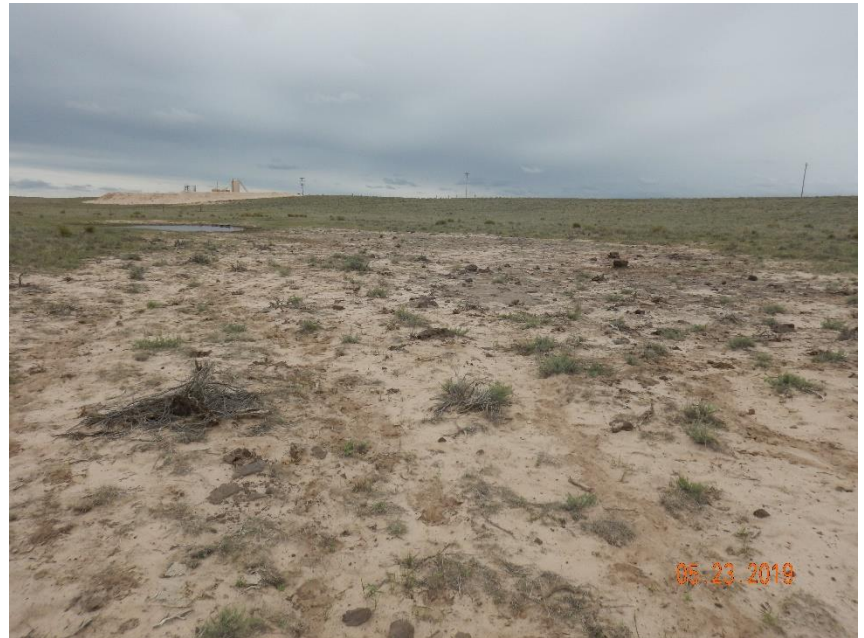
Photo 10: Photo taken from the east of the pits, facing north. Photo shows unvegetated areas where stained/contaminated soils are also evident. Aerial imagery suggests possible historic spill or discharge from pits.
