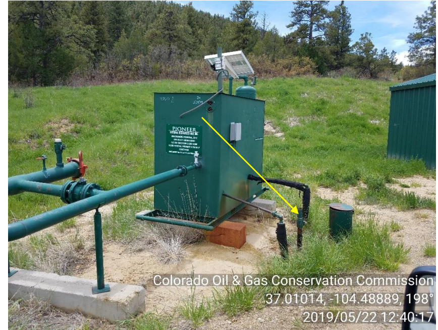
PHOTO 2: WELL SIGN POSTED DOES NOT DEPICT THE CURRENT OPERATOR. COMPLY WITH RULE 210. CA DATE 7/22/19. UNUSED EQUIPMENT UNMARKED UNUSED RISER NEAR METER HOUSE. COMPLY WITH 603.f. & NTO REGARDING UNUSED RISERS. CA DATE 7/22/19
