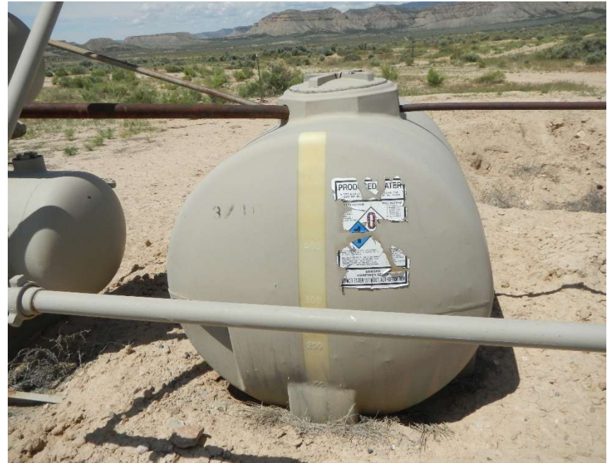
Photo #4 – NFPA placard on produced water tank (south of separator).
