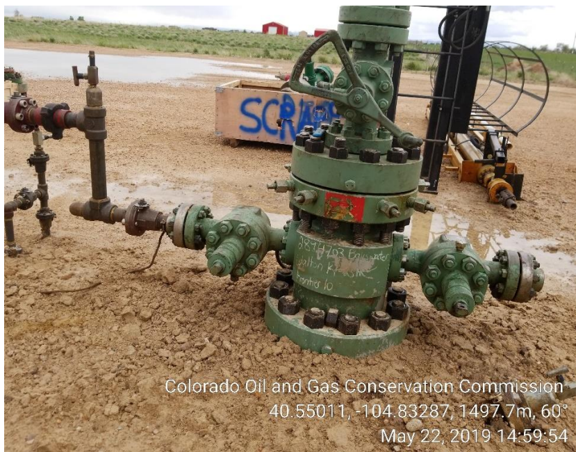
Photo 5: (TA) Wellhead; NO SIGN, UNUSED EQUIPMENT
