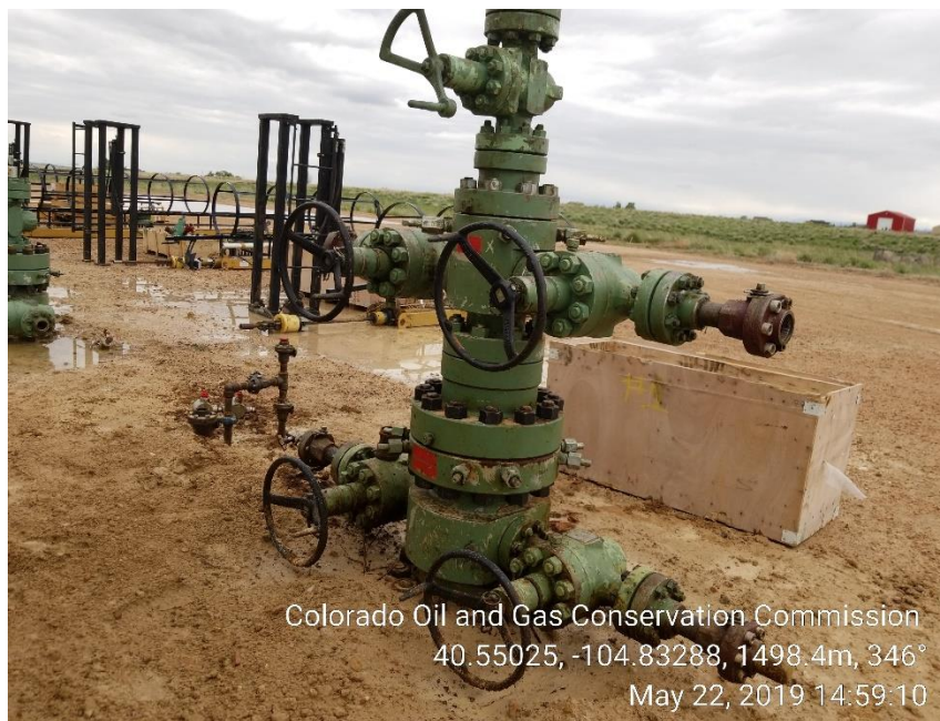
Photo 9: (TA) Wellhead; NO SIGN, UNUSED EQUIPMET
