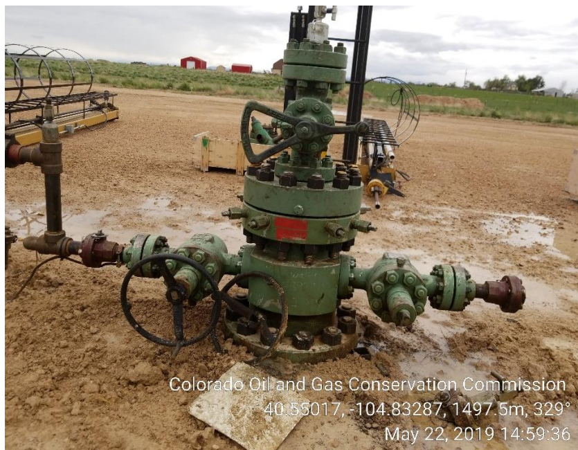
Photo 7: (TA) Wellhead; NO SIGN, UNUSED EQUIPMENT
