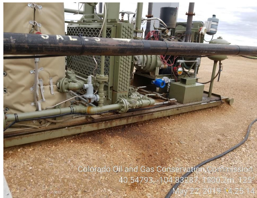
Photo 18: Stained soil east side of compressor
