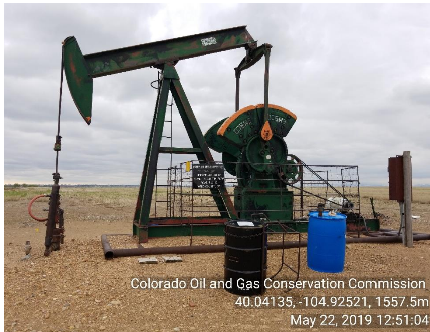
Photo 1 WH sign. Storm water improper storage of chemicals.
