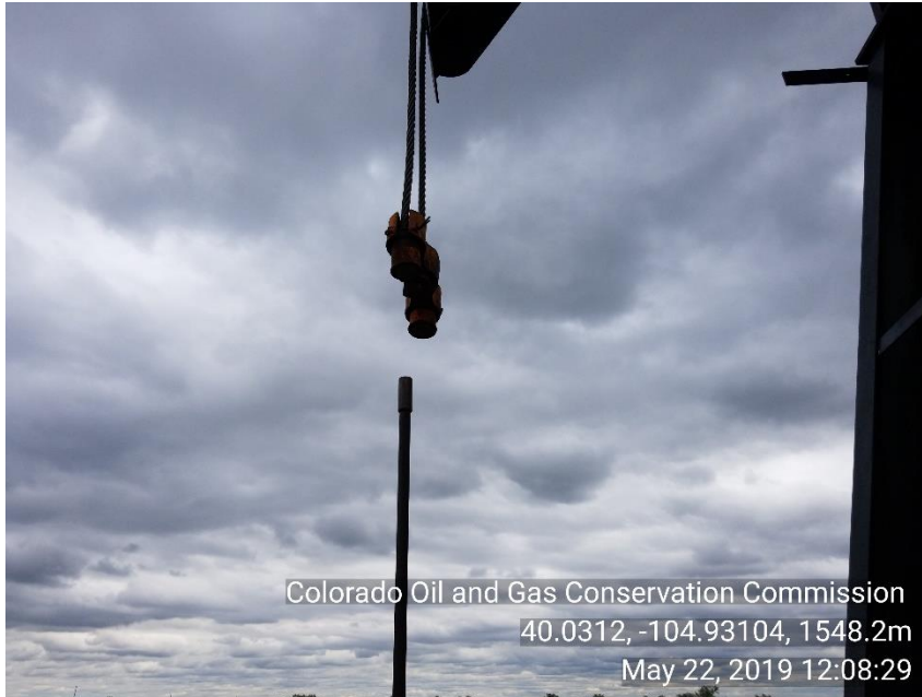
Photo 2 Horses head bridle not attached to rods.
