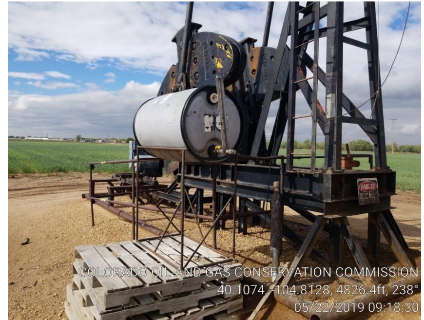
Pic 6 chemical tank with no containment no placard.
