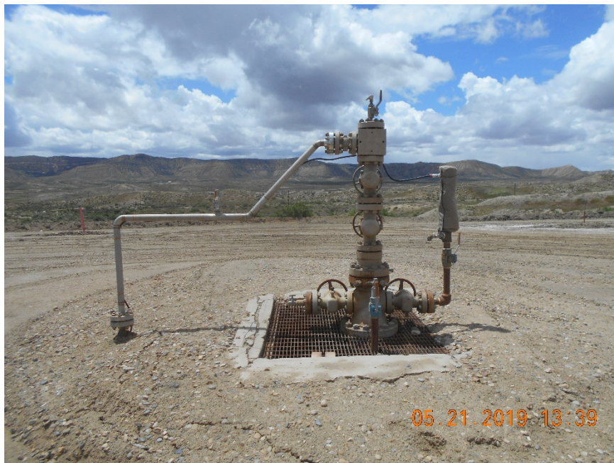
Injection wellhead
