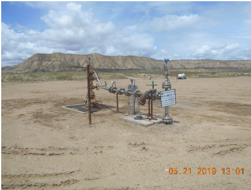
Injection wellhead
