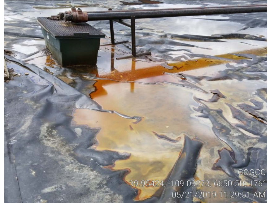
Photo 3. Oil sheen on water at tank off loading.
