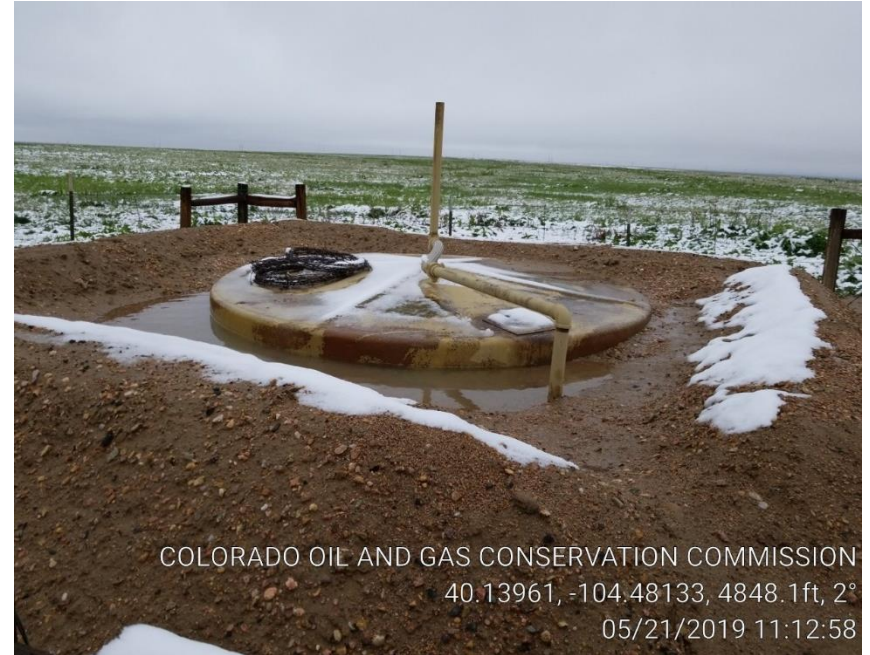
Pic 10 tank with no content label, capacity, or NFPA
