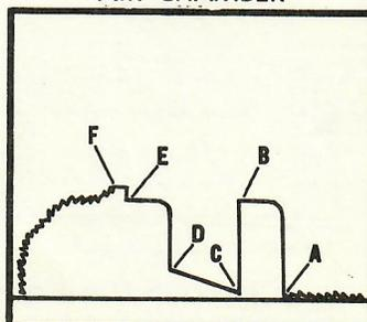
In this case a recorder has been run in an air chamber. The hydrostatic mud pressures are not influencing the recorder while going in or coming out of the hole due to the main tester valve being closed. The flow pressures and shut-in pressures are recorded while the main tester valve is opened.
