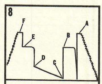
The packer has been unseated. The testing assembly is being removed from the hole.
