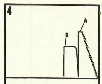
The chart indicates a pressure drop. The test tool has been opened to the surface either by breaking a disc, rotating a shut-in tool open or by reopening the main testing valve to permit the formation to produce.
