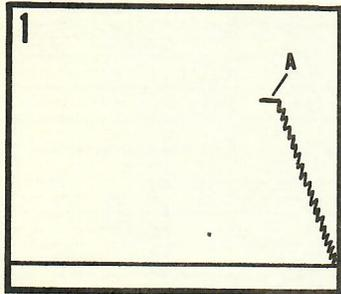
The pressure chart records the build-up in hydrostatic pressure as the testing assembly is lowered into the hole. Upon reaching the testing depth the hydrostatic head or pressure of mud column is recorded.
