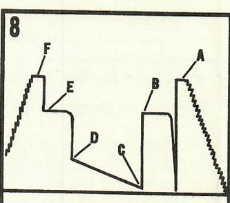
The packer has been unseated. The testing assembly is being removed from the hole.
