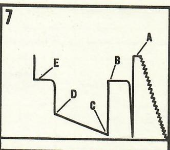
The chart shows the equalizing; the bypass ports have been opened permitting the drilling fluid to flow through the packer to the test zone. Thus, pressure is equalized above and below the packer. The equalization of the pressure facilitates easier removal of the packer from the packer seat.
