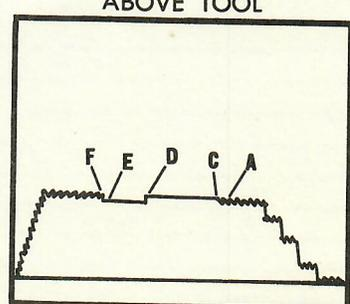
In this case a recorder has been run above the main tester valve with a fluid cushion used in the drill pipe. No pressure is recorded as the testing tool is being lowered into the hole. Then the fluid cushion pressure is recorded as the drill pipe is filled with fluid. As more stands are run into the hole, the recorder registers the hydrostatic pressures of the cushion. When the main testing valve is opened the pressure of the cushion column or the flowing pressure of the formation,
