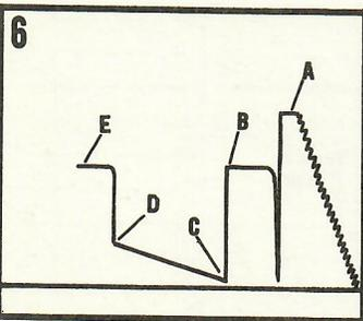
The final shut-in pressure is taken by stopping the flow of formation fluid into the drill pipe. Note the characteristic build-up curve. The well bore pressure is approaching equilibrium with the static reservoir pressure. When the shut-in curve levels-off the static reservoir pressure has been reached.
