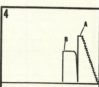
The chart indicates a pressure drop. The test tool has been opened to the surface either by breaking a disc, rotating a shut-in tool open or by reopening the main testing valve to permit the formation to produce.
