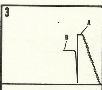
This chart shows the initial shut-in pressure. The methods by which this pressure can be taken allow only a minimum of formation fluid to be produced. This initial shut-in pressure is the best method yet devised for recording the original, undisturbed reservoir pressure of a formation.
