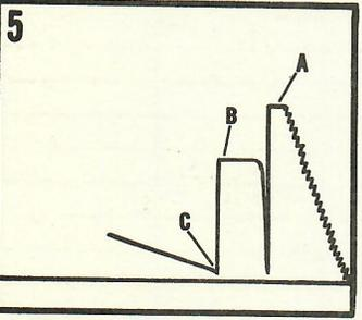
The pressure of fluid flowing from the formation into the well bore, through the perforated anchor, and into the drill pipe, is recorded on the chart.
