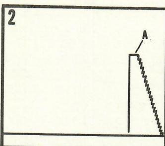
The packer is expanded and set to isolate the test zone. When the test valve is opened, a pressure drop is indicated on the pressure chart. This pressure drop is caused by removal of the hydrostatic mud pressure from the formation, allowing the formation to produce.
