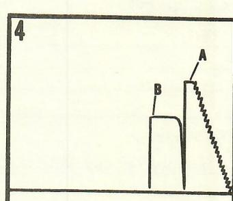
The chart indicates a pressure drop. The test tool has been opened to the surface either by breaking a disc, rotating a shut-in tool open or by reopening the main testing valve to permit the formation to produce.
