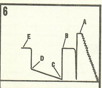
The final shut-in pressure is taken by stopping the flow of formation fluid into the drill pipe. Note the characteristic build-up curve. The well bore pressure is approaching equilibrium with the static reservoir pressure. When the shut-in curve levels-off the static reservoir pressure has been reached.
