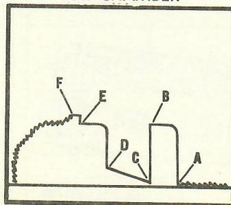
In this case a recorder has been run in an air chamber. The hydrostatic mud pressures are not influencing the recorder while going in or coming out of the hole due to the main tester valve being closed. The flow pressures and shut-in pressures are recorded while the main tester valve is opened.
