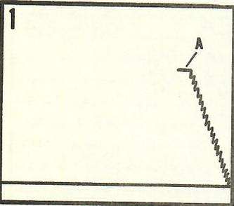
The pressure chart records the build-up in hydrostatic pressure as the testing assembly is lowered into the hole. Upon reaching the testing depth the hydrostatic head or pressure of mud column is recorded.
