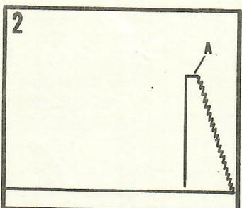
The packer is expanded and set to isolate the test zone. When the test valve is opened, a pressure drop is indicated on the pressure chart. This pressure drop is caused by removal of the hydrostatic mud pressure from the formation, allowing the formation to produce.
