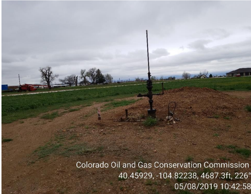
Photo 1 – Wellhead, still missing Wellhead Signage Info and Emergency Contact Info
