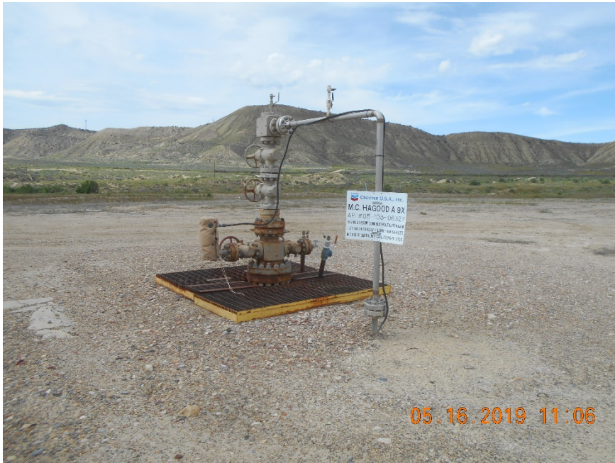
Injection wellhead
