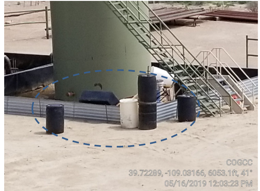
Photo 11. Unlabeled containers stored without secondary containment.
