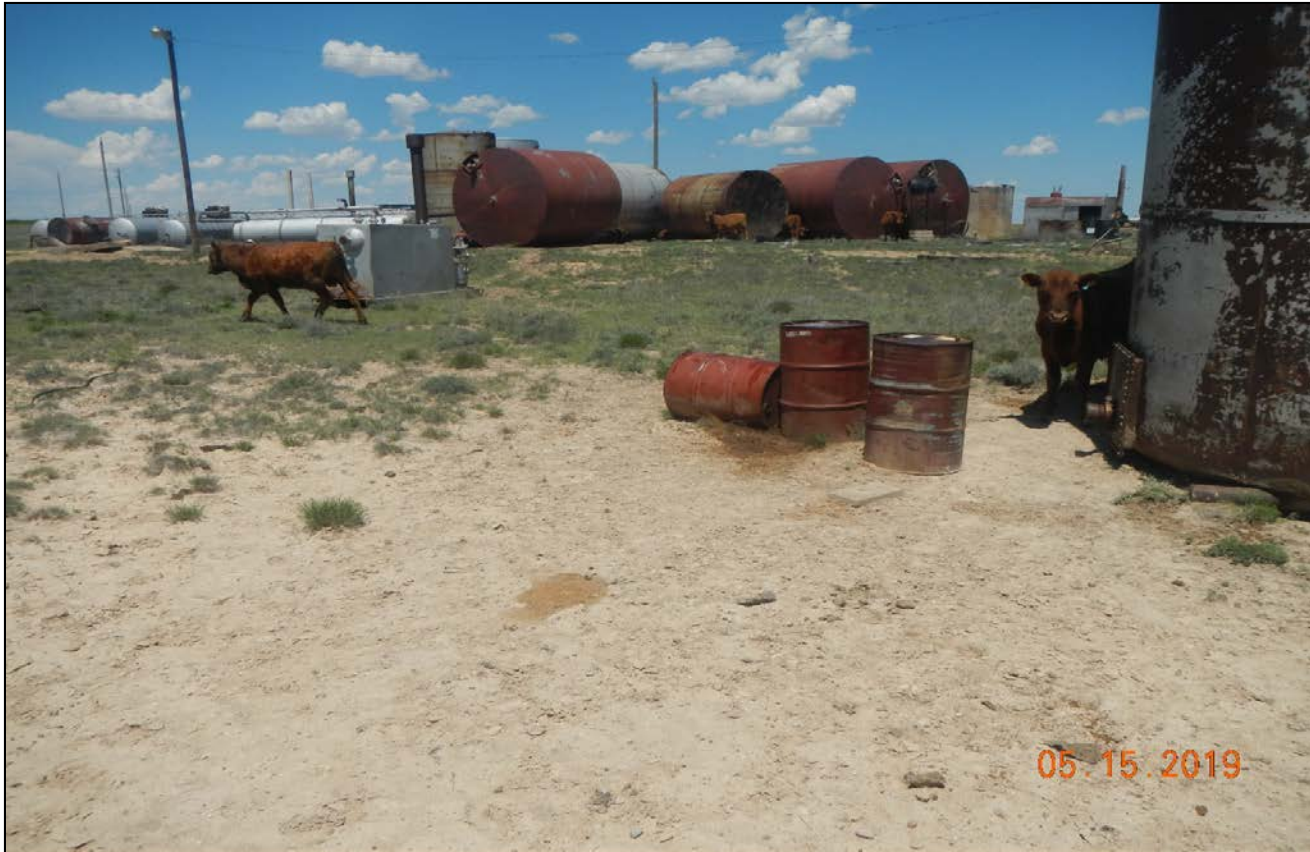
Photo 10. Facing toward the unused equipment. There are barrels with what appears to be oil with no labeling or containment. One barrel is tipped over with oil stained soil from spillage.
