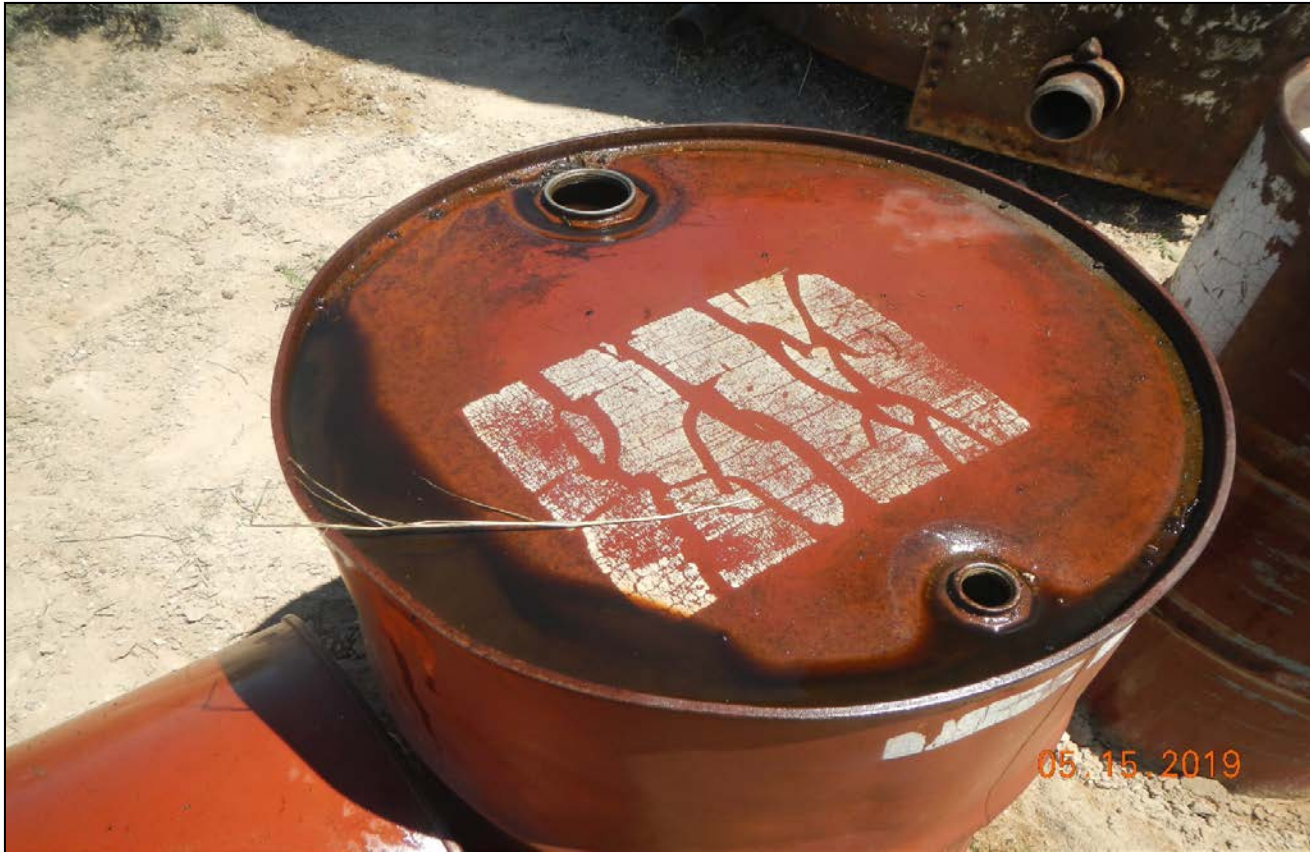
Photo 11. The barrels appear to full of oil with no cap and there is oil on the top surface.
