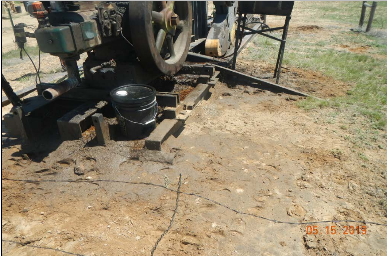
Photo 6. There is oil stain soil around the pump jack. There is a 5 gallon bucket with no labels or secondary containment.
