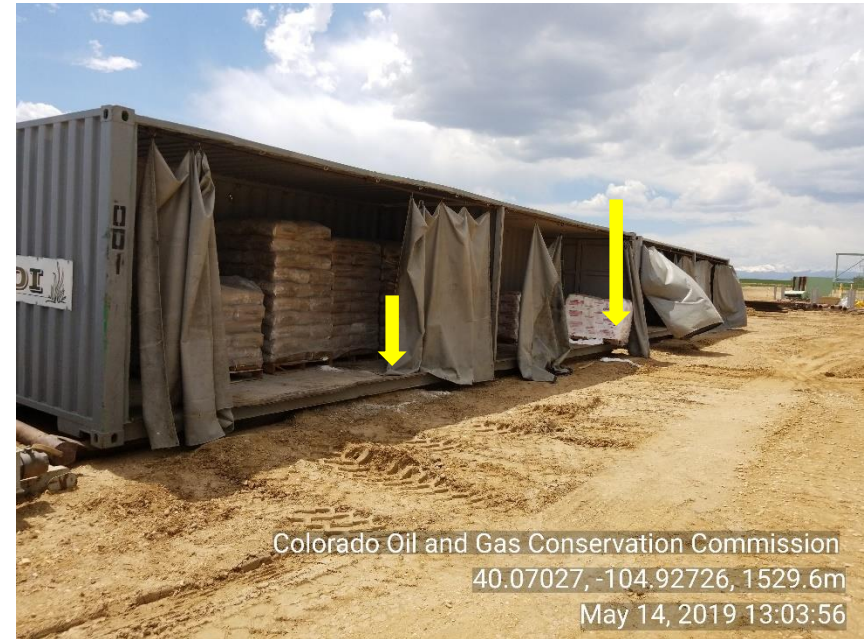
Photo 10 Chemical storage. Chemical's appear to have spilled outside containment.
