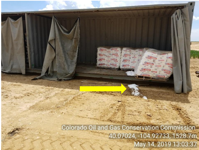
Photo 9 Improper chemical Handling
